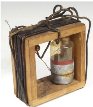
LEFT: Marconi's First Tuned Transmitter: a tuned circuit with insulated cable wound around a square dovetailed wooden frame containing a Leyden jar and brass-ball spark gap.
