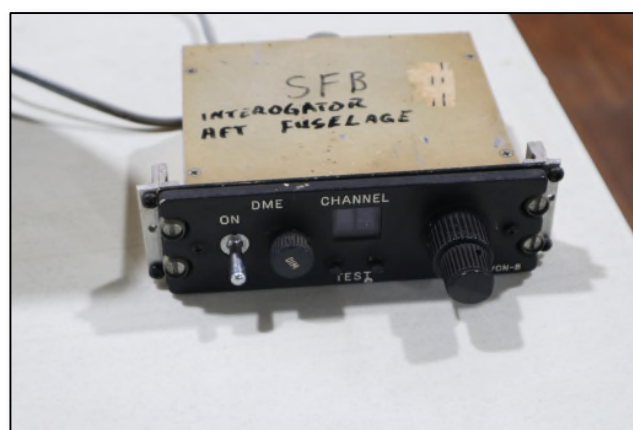
Above: The Australian designed aircraft "distance measuring equipment (DME) was used worldwide.
