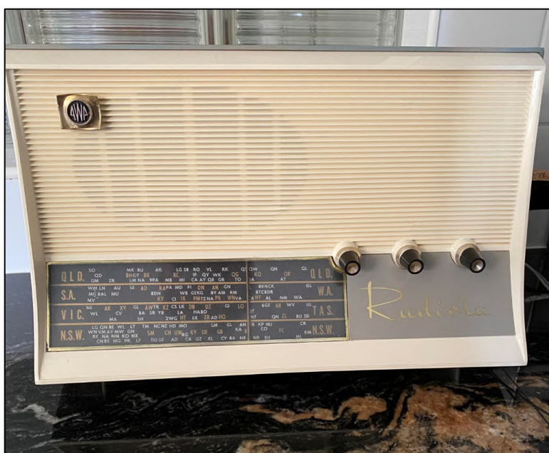
Above: From 1966 – The uniquely designed AWA B-15 was one of the last 5-valve mantle radios. Using the same chassis and case, AWA developed an all-transistor portable model, the B-23. This one was badly damaged and has been extensively restored.
