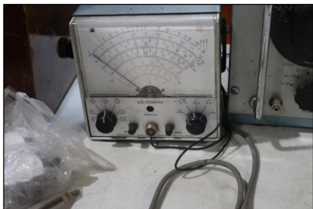
Above: John's AWA VOLTOHMYST – A versatile instrument, used to measure both +ve and -ve DC voltages; DC current, resistance and AC voltages.
