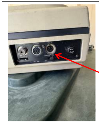
Socket for 12volt push-in power lead.
