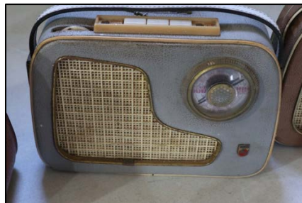
Above: A pair of Philips model 196A portable radios – Made by Philips at Hendon in 1959. These are AC/DC powered models, and were the last all-valve portables.
