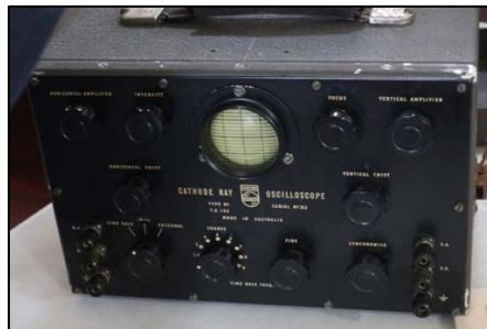
Above: Peter Holland's TA155 (1948) model Phillips Cathode Ray Oscilloscope with a 2 inch diameter screen.
