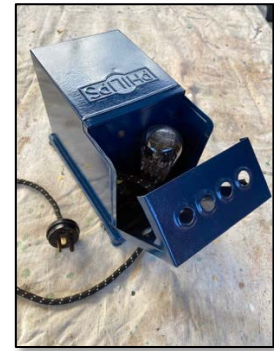
Above: Ian Smyth's fully restored Philips "Battery Eliminator" (Uses a 506 valve as rectifier.)
