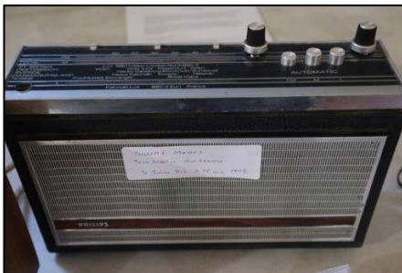
Above: Philips (1968) 22RL383/00R Made for European market, it received LW/MW/FM bands. Used 6 x 1.5v batteries.
