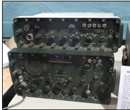
Above: Tony Bell's R5223 HF Receiver set – designed for surveillance and field communications. Made at Philips Hendon factory in 1960's.
