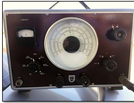
Above: Philips GM2317 Audio Signal Generator. Rescued from Philips factory and now fully restored.
