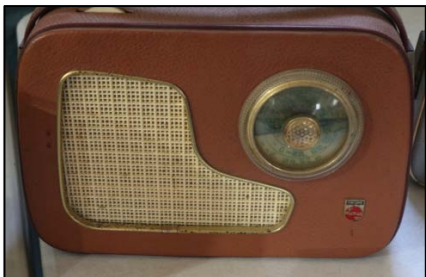
Above: A pair of Philips model 196A portable radios – Made by Philips at Hendon in 1959. These are AC/DC powered models, and were the last all-valve portables.
