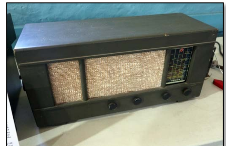
Above: John Crawford's Philips 3250W (1943) "Amenities" radio. Sold through Amenities shops for military personnel. Used a 6v synchronous vibrator.
