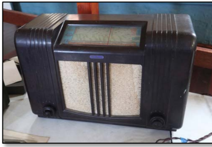
Above: Colin Windsor's fully restored 6v vibrator powered Mullard model MBV-1102 "farm radio". Made by Philips. (1948)
