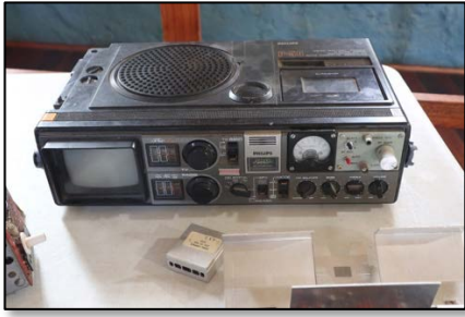
Above: Philips P-50 AC/DC battery powered 3-band radio & monochrome TV with cassette recorder
