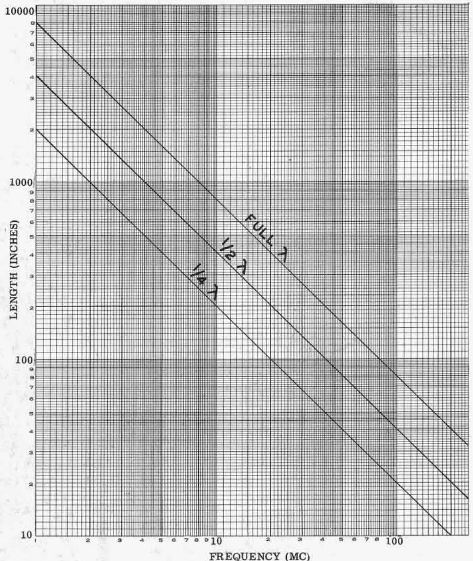
Figure 1. Wave length vs frequency for coaxial cables having polyethylene dielectric.
