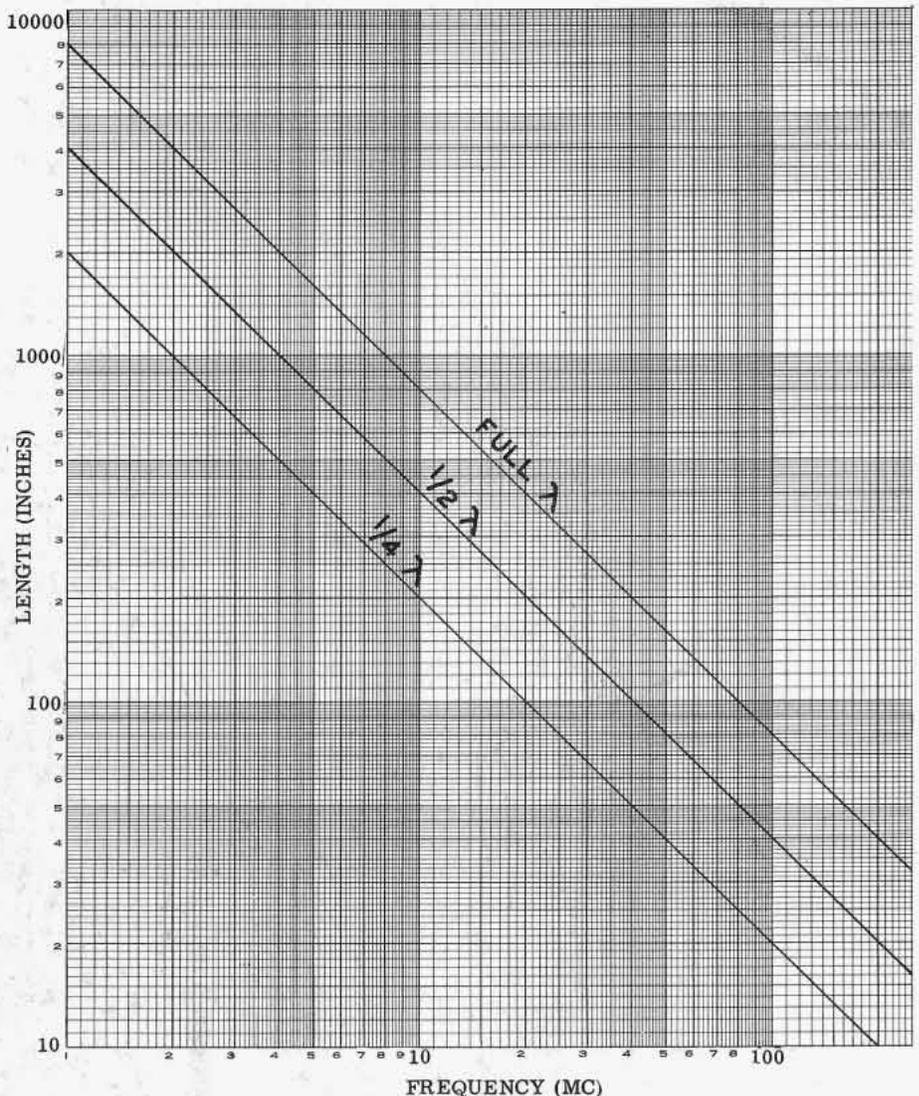
Figure 1. Wave length vs frequency for coaxial cables having polyethylene dielectric.
