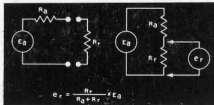
Figure 1. I.R.E. Standard for introducing signal voltage  $E_a$  through antenna impedance  $R_a$  into receiver input impedance  $R_r$ .
