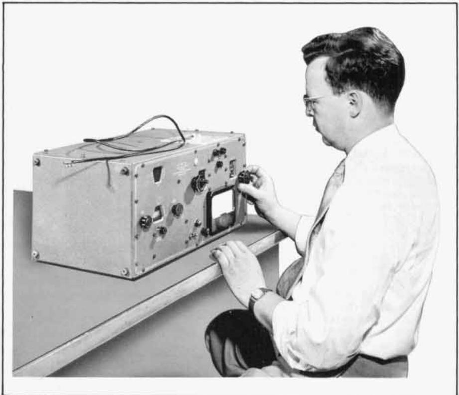
Figure 2. The author, measuring the characteristic impedance of a short length of RG-58/U cable on the RX Meter.
