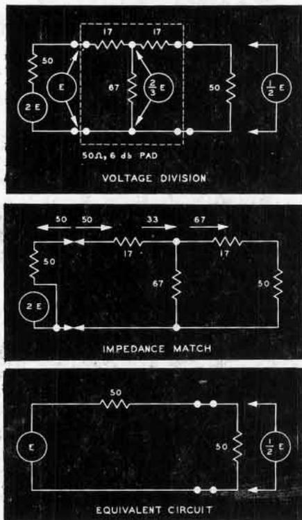
Figure 5. Equivalent circuit of a 50-ohm, 6 db symmetrical attenuating pad.
