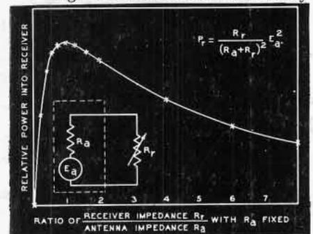
Figure 2. Effect of variation of receiver input impedance  $R_r$  on power into receiver with fixed antenna impedance  $R_a$  and voltage  $E_a$ .
