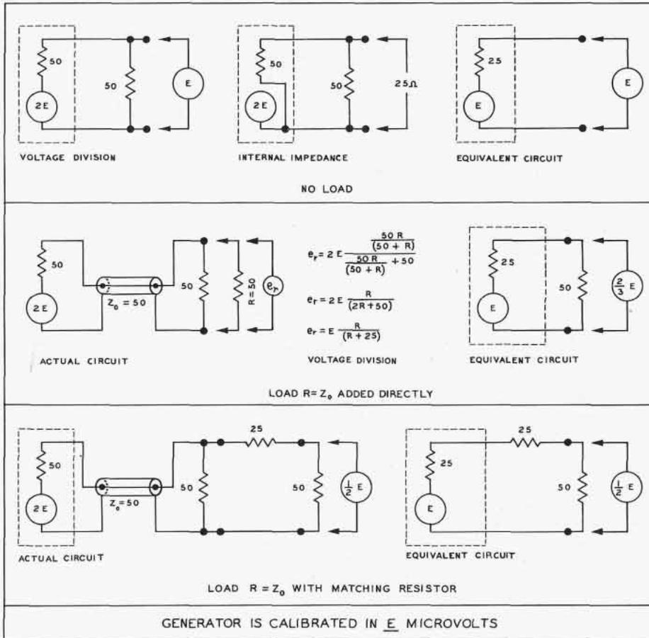
Figure 4. Application of Thevenin's Theorem to a cable terminated in  $Z_0$ .
