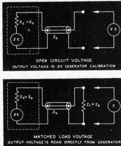
Figure 3. Output voltage calibration for a generator having its source impedance equal to the characteristic impedance of the output cable.
