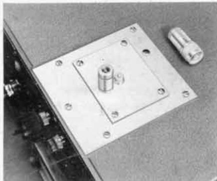
Figure 2. The Co-ax Adapter, mounted on an RX Meter. The 50-ohm termination shown beside the terminal plate is used in obtaining preliminary balance of the RX Meter bridge circuit.
