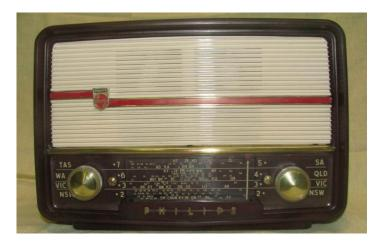
This is a Philips Model 167, which was brought to me by a collector, who had replaced the capacitors including the two electrolytics, but when it was powered up, R12 became so hot that it smoked!
