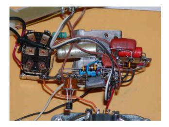
The transistor is in a socket to allow for easy experimentation and is optional. Except for the transistor, the component values and types are pretty forgiving so substitutions may work fine.
